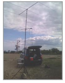
Below are the totals from the CQ WW VHF contest this weekend along with a snapshot of the operating position taken late in the day with the camera in my iPhone. (It was pretty badly backlit so I cranked up the brightness.) The top antenna is a 6m Buddipole beam with an eight foot boom and three elements. The bottom antenna is an Arrow handheld antenna with the optional mount clamped to the Buddipole mast. Both antennas performed very well.
