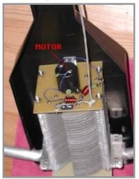
I guess you can file tonight's entry under, "I really didn't need any more problems, but..." The MFJ loop I've been using died again. Specifically, the small 1 RPM motor in the unit stopped working. This is the second replacement motor I've installed. The first, luckily, died while the unit was under warranty. And, true to MFJ's word, they sent me a free replacement quickly with no questions asked. This one was, now that the unit is out of warranty, \$40. {sigh}
