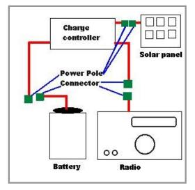
Every interconnect of power was with a mated set of Power Poles. The solar panel has a Power Pole, the charge controller has *3* (one for connection to the solar panel, the battery, and to the load/radio), and the batteries I have along with the power cords for the radios are all terminated with a Power Pole connector. If I need to swap out the battery, just pull apart the connection and insert the Power Pole connector from the new battery. Easy!
